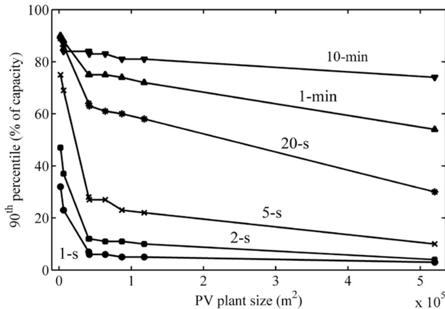
Figure 1. 90<sup>th</sup> percentile of step changes in the output from differently sized PV plants, based on values reported in Marcos et al. (2011a).
