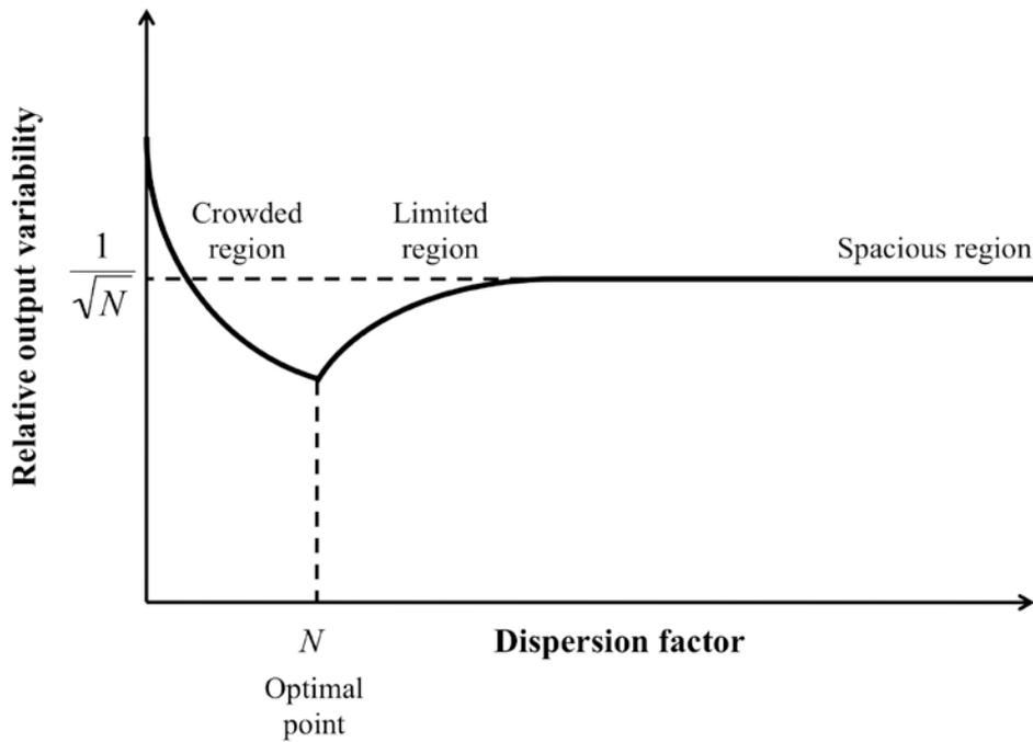
Figure 2. Schematic outline of the relative output variability as a function of the dispersion factor, with the different regions in the Hoff and Perez model indicated. Based on a similar outline in Hoff and Perez (2010).
