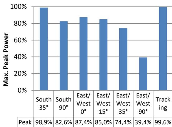
Figure 7. Maximal peak power rated to nominal power
