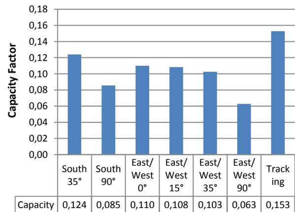
Figure 2. Capacity Factor
