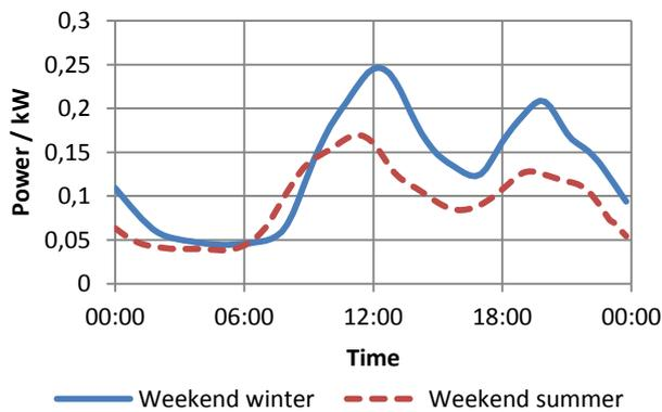
Figure 4. Typical residential customer load profile (H0-Profile)
