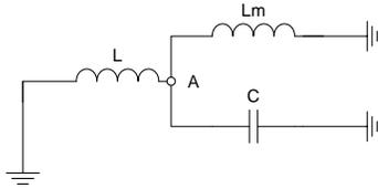
Fig. 6. Simplified example for motor load impact
