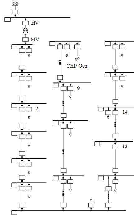
Fig. 2. Medium voltage part of the example network
