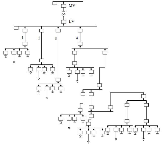
Fig. 1. Low voltage part of the example network
