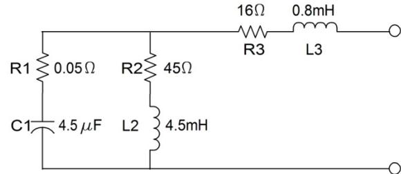
Fig. 9. The impedance model of TP inverter.
