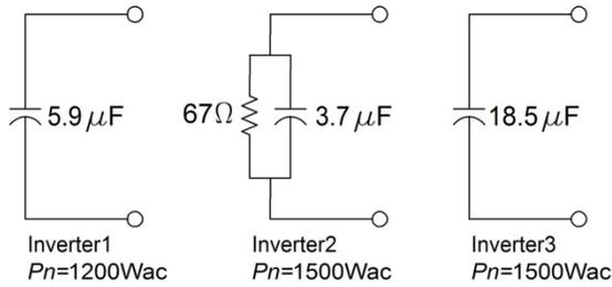
Fig. 6. The impedance models of SP inverters.
