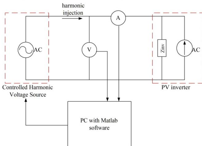
Fig. 2. Measurement schematic.
