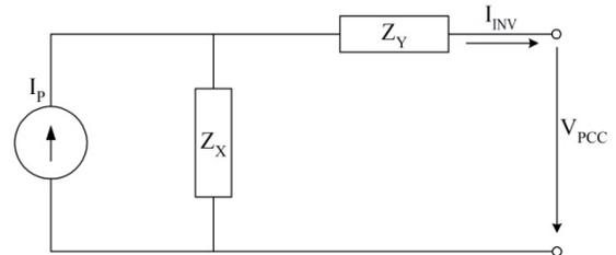
Fig. 1. An impedance and current source circuit as PV inverter model.
