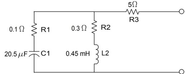
Fig. 8. The impedance model of SP power router.
